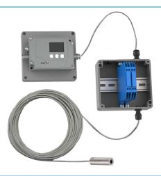
EL50-HEx is a digital Pyrometer in economic range with extended sensor head in 4 wire technology, for non-contact temperature measurement between  $0^{\circ}\text{C}$  to  $800^{\circ}\text{C}$ . The sensor head is unaffected by electromagnetic interferences. The pyrometer sensor head is specially designed to withstand ambient temperature upto  $180^{\circ}\text{C}$  without cooling.
