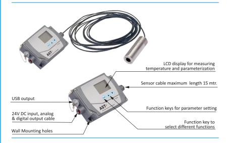
EL50-H+ is a digital Pyrometer in economic range with extended sensor head in 4 wire technology, for non-contact temperature measurement between 0°C to 800°C. The sensor head is unaffected by electromagnetic interferences. The pyrometer sensor head is specially designed to withstand ambient temperature upto 250°C without cooling.
