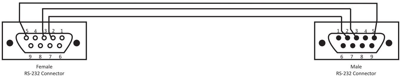
Fig. 23 Serial Communication Cable Male/Female (RS-232 Communication Cable)
