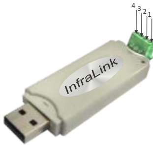
Fig. 17 Infralink USB interface (Reference no: 9000-07 )
