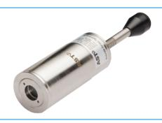
IR-CAST 2C is a highly accurate digital two colour Rectangular measuring field IR pyrometer for non contact temperature measurement specially used in foundries for molten metal. The Pyrometer measures the temperature of an object by calculating the ratio of the energies at two different wavelength bands. The ratio technique eliminates and reduces errors in temperature measurement caused by factors such as dust, vapour or smoke etc.
